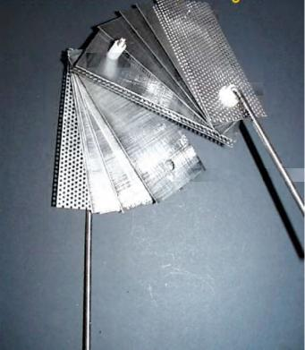
Next, leaving all but the starting nuts loose, the two halves can now be assembled to make the entire unit. I have to stress this issue about tubings that need to end against a nut & washers that slip over tubing need to do just that, because they can & will move untill put in their correct order upon tighting the final nuts. Cut plastic tubings to leave enough thread to allow a nut & washer, plus a little at each of the ends.
